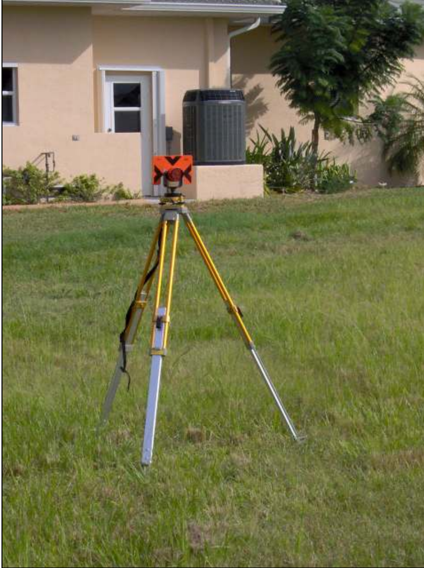
Figure 4.2: Reflector Used as a Reference Point for the EDM
